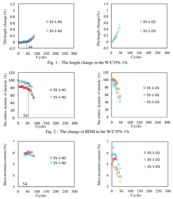
Fig. 3 – The change of mass moisture content in the W/C35%-1%
